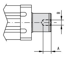
The inside thread option comes mounted from factory if this is stated in the ordering key at order. Possible types for the different unit sizes depend on the ball screw diameter of the unit, see "Ball screw diameter" in the table.
