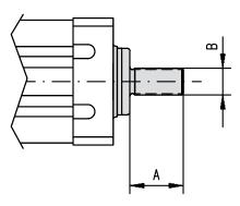
The outside thread option comes mounted from factory if this is stated in the ordering key at order. Possible types for the different unit sizes depend on the ball screw diameter of the unit, see "Ball screw diameter" in the table.
