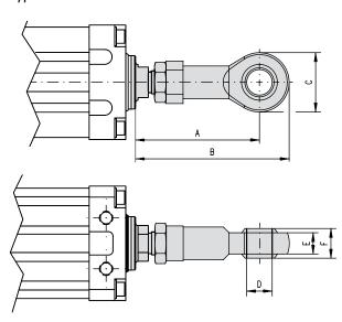
The spherical joint option can be mounted on the unit from the factory if this is stated in the ordering key at order, or can be ordered separately using the part number(s). When ordered separately, all necessary components to attach the spherical joints to the unit are included. Type M joints include a grease nipple. Note: When ordering a spherical joint separately, make sure that the extension tube end has an outside thread adapter to be able to mount it.
